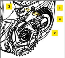
Chainguide – use only with positive foot-retention devices on the pedals
